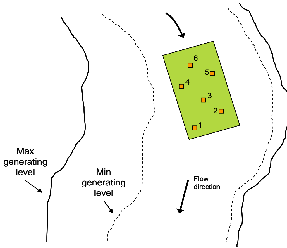
Figure 3. Overhead view of a site (green rectangle) and sampling locations (orange squares) in relation to maximum and minimum generating levels.
